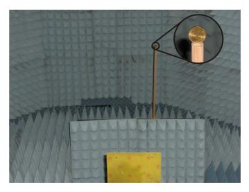
Fig. 16. Measurement setup using a 50-cent Euro coin as target. The used coin has a diameter of 24.25 mm and was placed at a distance of 1.7 m to the radar.
