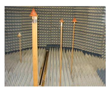
Fig. 20. Measurement setup used for moving target measurements. The photograph was taken at the beginning of the target movement and shows the case where three CCs are static, whereas one is mounted on a rail and moving.
