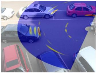
Fig. 24. Photograph of the measurement scenario on a parking lot with multiple cars overlaid with the calculated power distribution (cf. Fig. 23). The sundry scattering centers of the different cars can clearly be observed and related to different parts of the cars.
